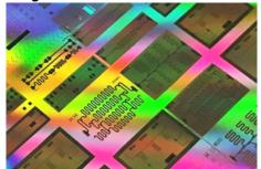
Test chip with superconducting qubits in a 300 mm integrated process prototype. (© IMEC)
