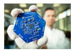
The self-sufficient sensor node developed in project ZEPOWEL falls into deep-sleep mode when it is not needed. © Fraunhofer IZM, Volker Mai.
