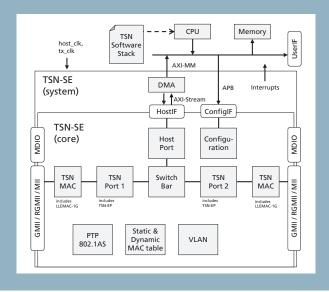
Schematic diagram of the TSN-SE IP Core.
