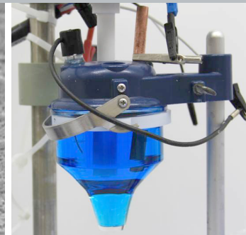
▲ Cyclovoltammetric measurement setup including copper electrolyte
