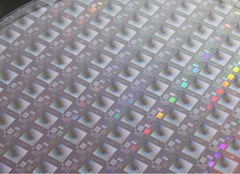
300 mm CMP test wafer with pitch / density structures down to 28 nm node
