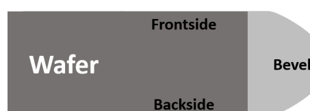
Scheme illustration of the wafer side view
