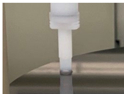
Nozzle fixating the droplet while wafer underneath rotates performing a surface scan
