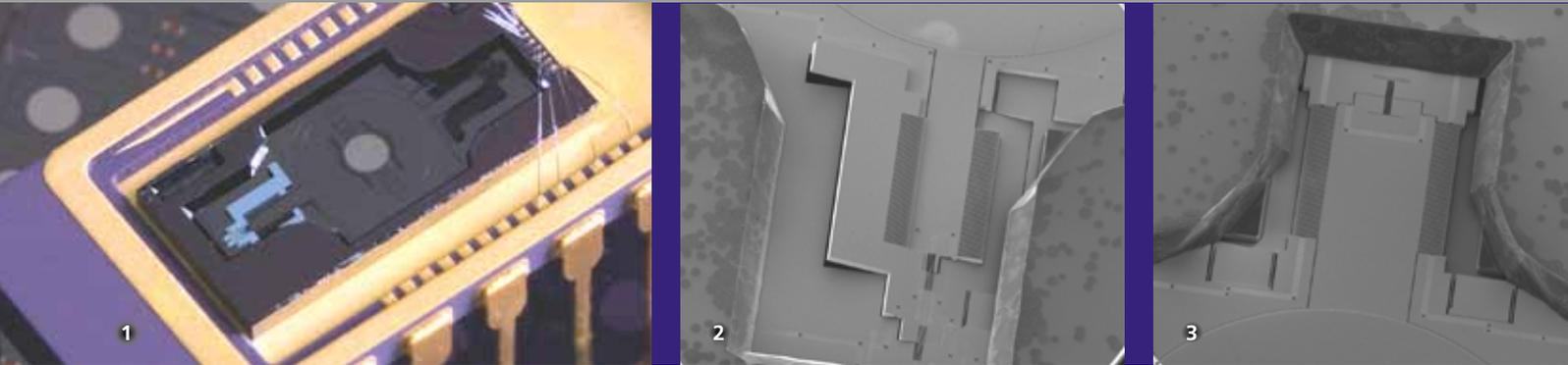
1 2D LinScan microscanner demonstrator in DIL20 ceramics housing.
