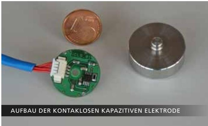
AUFBAU DER KONTAKLOSEN KAPAZITIVEN ELEKTRODE
