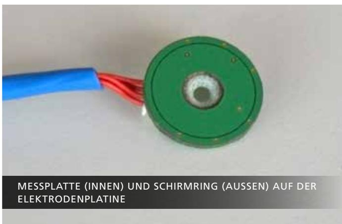
MESSPLATTE (INNEN) UND SCHIRMRING (AUSSEN) AUF DER ELEKTRODENPLATINE
