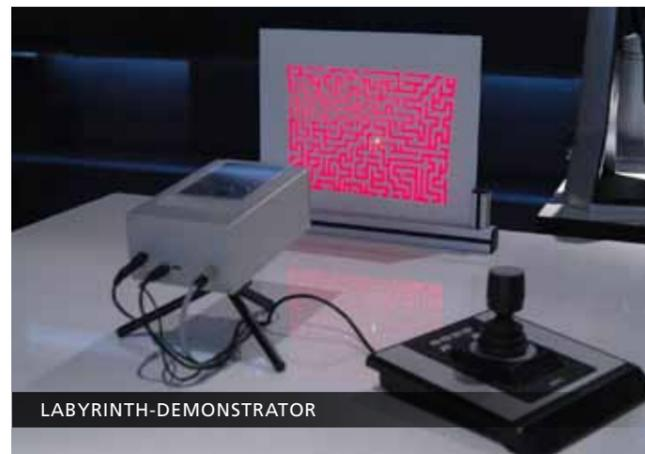
is deflected by two quasi-static microscanners and is controlled with a joystick. Both demonstrators, which generated a lot of interest at the trade show, are the result of an internal idea competition for show exhibits which was held by the Institute in the first half of 2012.
