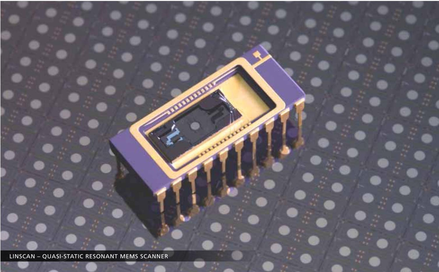
Fraunhofer IPMS has been working on scanning mirrors that deflect light in one and two dimensions for years. Up until now, the components that have been field-tested in numerous customer projects could only resonate continuously at one set frequency. A new concept for a quasi-static scanner – called LinScan – now makes the variable adjustment of the motion pattern possible, opening up new application possibilities.
