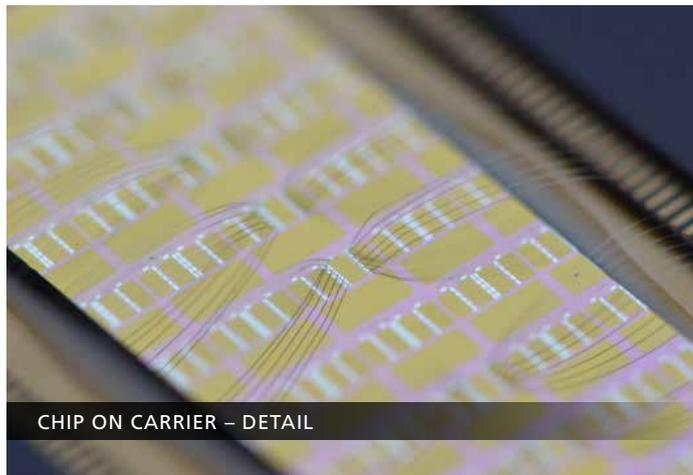
The first generation of Fraunhofer IPMS’ CMUT arrays is currently being characterized. In addition to the optical inspection and X-SEM images, white light interferometry was performed to check on the homogeneity of the CMUTs within CMUT group to wafer location dependency.
