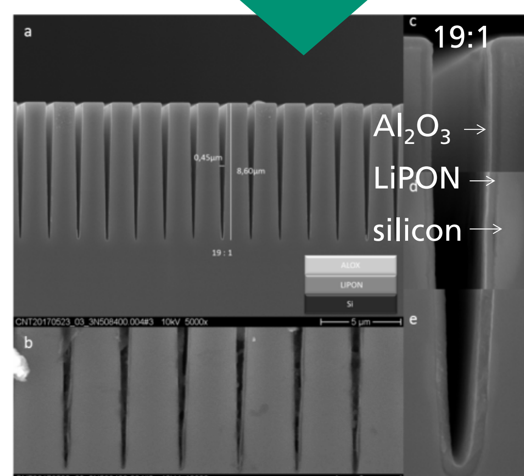
Fig. 1 ALD electrolyte LiPON with protecting Al 2 O 3 capping in trenches
