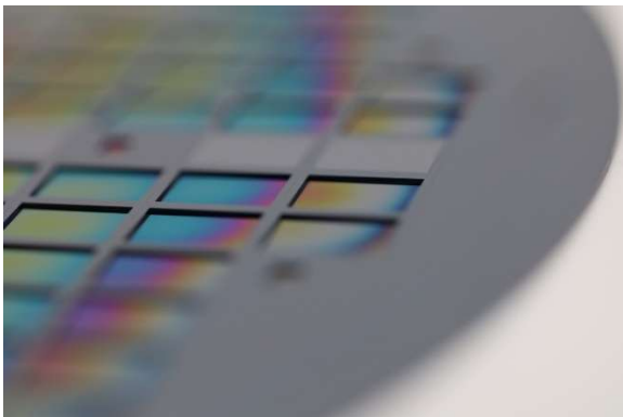
Wafer with placed chiplets © Fraunhofer IPMS
