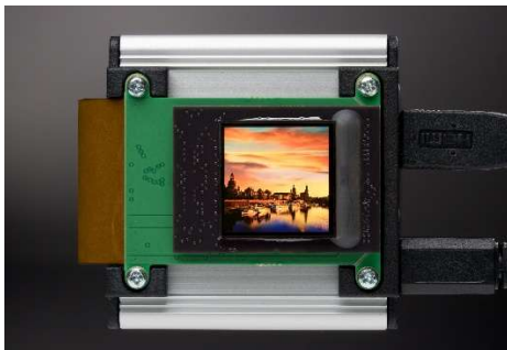
OLED microdisplay with 2K resolution (2,048 × 2,048 pixels, 1.07 inch).
