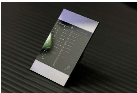
A miniaturized photonic biosensor chip developed by Fraunhofer IPMS using integrated photonics.
