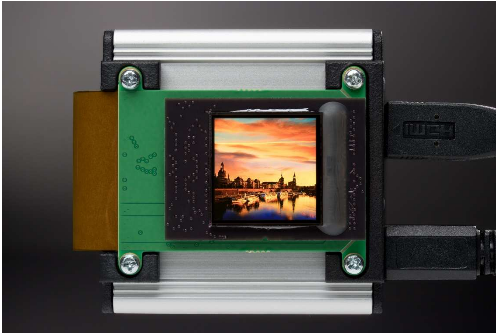
OLED microdisplay with 2K resolution (2,048 × 2,048 pixels, 1.07 inch). © Fraunhofer IPMS
