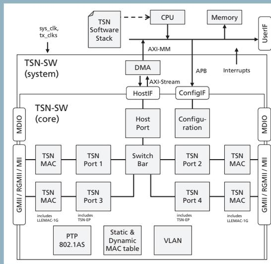
Schematic diagram of the TSN-SW IP Core.
