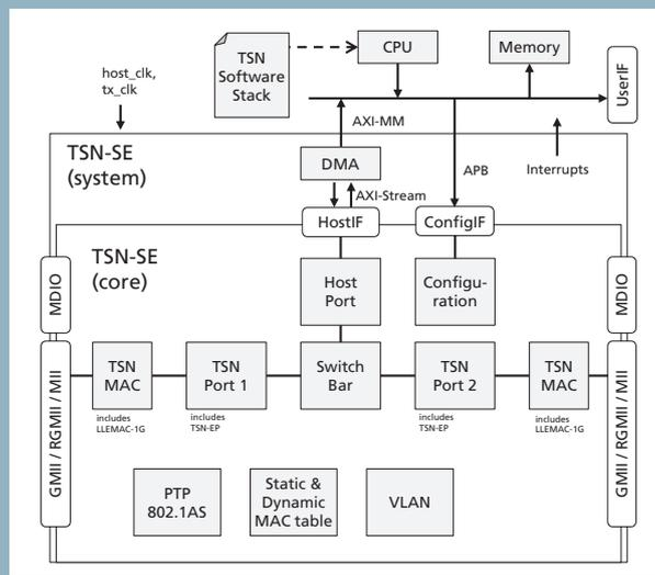
Schematic diagram of the TSN-SE IP Core.
