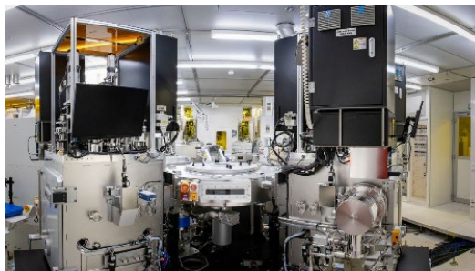
The new tools enable the thermal deposition of complex organic stacks, metal layers, and oxides, facilitating the development and manufacture of high-resolution OLED microdisplays as well as sensors such as organic photodiodes. © Fraunhofer IPMS
