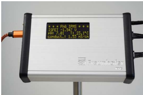
Multi-Sensor System: Sensor control for recording and displaying measurement data. © Fraunhofer IPMS
