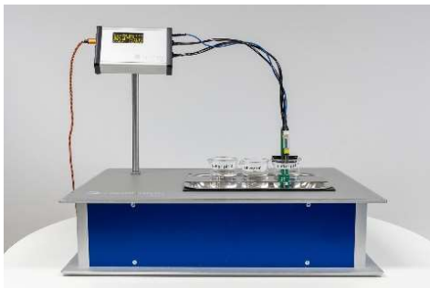
Demonstrator for pH and conductivity measurement © Fraunhofer IPMS
