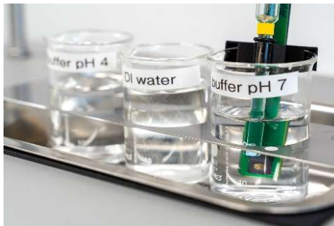
Exemplary measuring arrangement with ISFET, conductivity sensor and reference electrode © Fraunhofer IPMS
