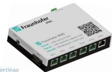
TSN Evaluation Kit: Xilinx ZCU102 or Intel Netleap (Cyclone V SoC); implemented IPMS TSN-IP core for switch applications (TSN-SW).
