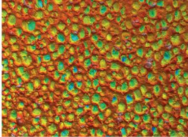
CMP pad pore structure obtained with confocal microscopy  $(0.7 \times 0.5 \text{ mm})$
