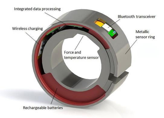
A self-organizing, user-oriented and demand-driven automated production (Industry 4.0) requires a large variety of connected, structure-integrated sensors. These devices must be robust, have a small form factor and should communicate wirelessly. A promising approach is the functional and structural integration of microelectronic and micromechanical devices and subsystems into the equipment.
