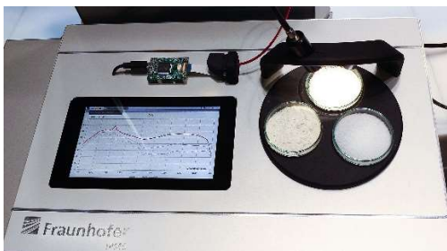
Demonstration system for spectroscopic identification of white powders. © Fraunhofer IPMS
