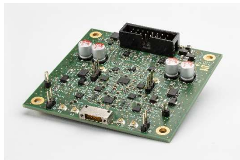
Drive electronics for electromagnetic vector scanners. © Fraunhofer IPMS
