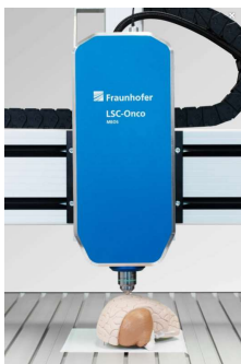
By using MEMS technology, the laser scanning microscope of the LSC-Onco project is so small and compact that it can be used directly on the patient in the operating room. © Fraunhofer
