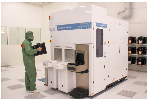
Applied Materials' eBeam metrology equipment at cleanroom of Fraunhofer IPMS © Fraunhofer IPMS
