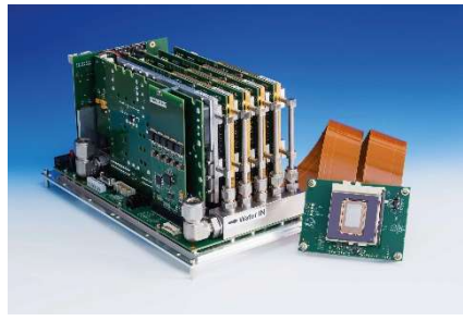
2-axis tilting mirror module of Fraunhofer IPMS; SLM chip with control electronics. © Fraunhofer IPMS
