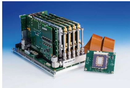
SLM chip with control electronics © Fraunhofer IPMS
