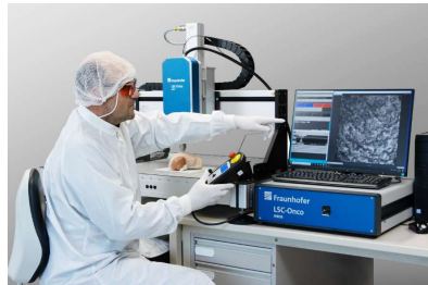
Laser scanning microscope for tumor delineation © Fraunhofer IPMS
