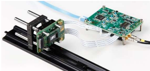
Customer Evaluation Kit for quasi-static MEMS scanners © Fraunhofer IPMS
