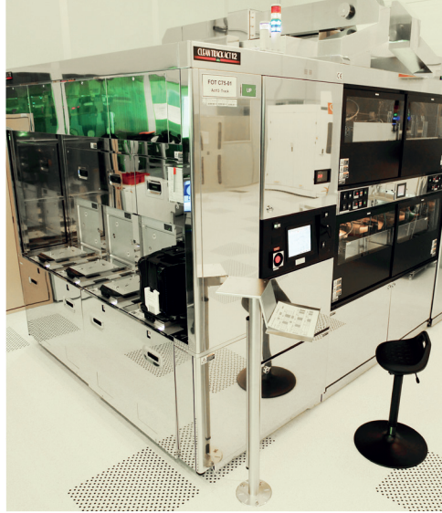
TEL ACT 12 Clean Track for fully automated 12" coating and development
