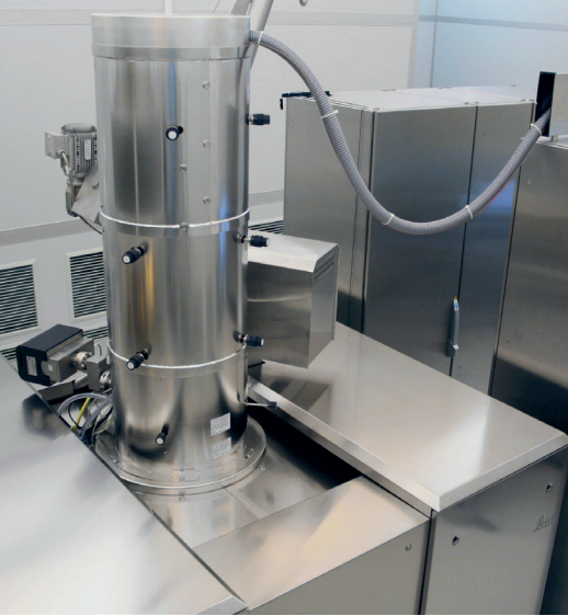
Vistec SB3050DW variable shaped E-beam for direct maskless patterning
